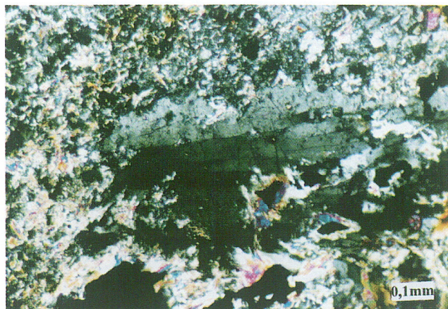
Fig. 9. Subhedral andalusite in macroscopically spotted andalusite hornfels. Borehole DB-5, depth 570.2 m; Crossed polars
