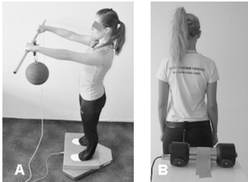
Figure 2. Assessment of postural and core stability using the FiTRO Sway Check system completed with a special program for Load Release Balance Test (a) and the FiTRO Dyne Premium system (b)
