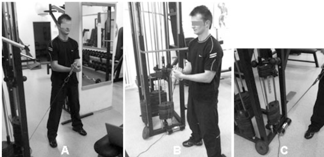
Figure 4. Measurement of strength parameters during the standing cable wood chop exercise on a weight stack machine (a, b) using the FiTRO Dyne Premium system (c).
