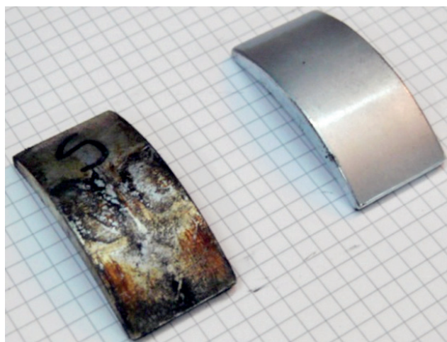
Fig. 14. N38UH magnets – a damaged magnet on the left, a new magnet on the right
