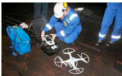
Figure 5. Tests in the Remontowa Shipyard by DNV-GL-tests with drones inside a tanker (poland@sea, 2016)
