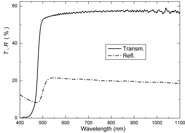
Fig. 2. The spectral dependence of transmittance and reflectivity for  $\text{Tl}_4\text{InGa}_3\text{S}_8$  crystal at  $T = 300$  K.
