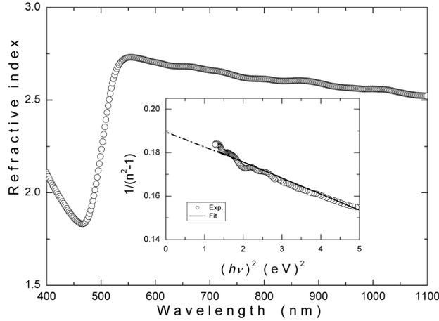
Fig. 5. The dependence of refractive index on the wavelength for  $\text{Tl}_4\text{InGa}_3\text{S}_8$  crystal. Inset: Plot of  $(n^2 - 1)^{-1}$  versus  $(h\nu)^2$ . The solid line represents the fit using Eq. (5).
