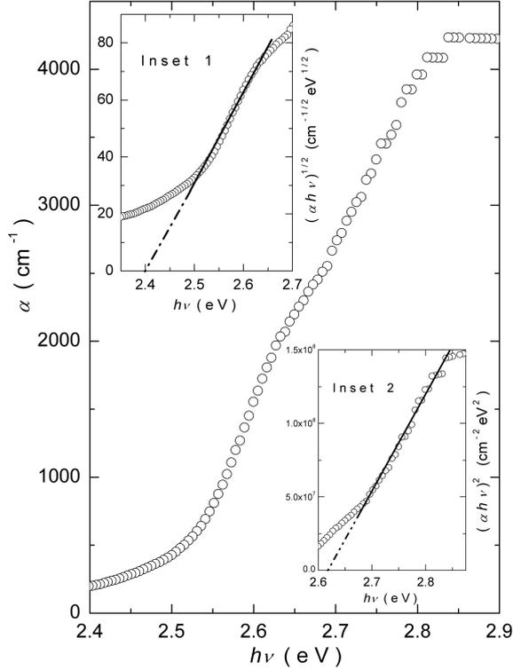
Fig. 3. The variation of absorption coefficient as a function of photon energy at  $T = 300 \text{ K}$ . Insets 1 and 2 represent the dependences of  $(\alpha h\nu)^{1/2}$  and  $(\alpha h\nu)^2$  on photon energy, respectively.
