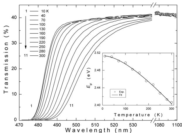
Fig. 4. The spectral dependence of transmittance for  $\text{Tl}_4\text{InGa}_3\text{S}_8$  crystal in the temperature range of 10–300 K. Inset: the indirect band gap energy as a function of temperature. The solid line represents the fit using Eq. (4).
