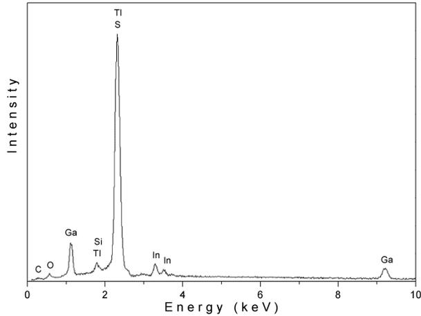
Fig. 1. Energy dispersive spectroscopic analysis of  $\text{Tl}_4\text{InGa}_3\text{S}_8$  crystal.
