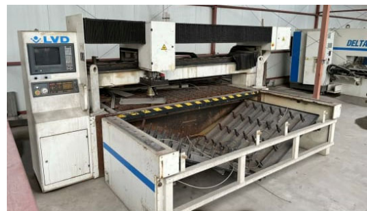
Fig. 2. The laser cutting machine LVD model (2513) is used in cutting stainless steel 2505
