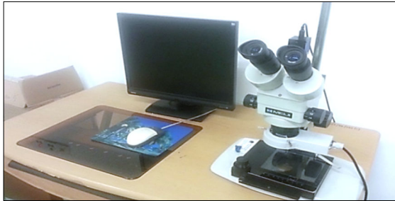
Fig. 3. Optical microscopy with (mag. 1.2x) used for measuring kerf width
