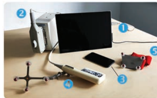
Figure 2. Components of the measuring system (1: Tablet Microsoft Surface Pro 4, 2: Ultrasound device, 3: iPhone 7, 4: Ultrasound probe and adapter with a marker, 5: Marker on a tape)
