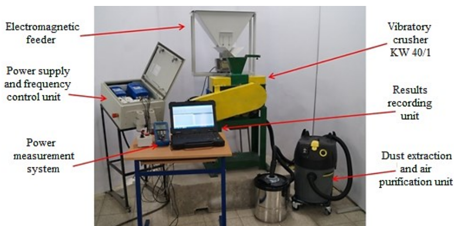
Fig. 1 View of the laboratory test station of the vibratory jaw crusher type KW 40/1
