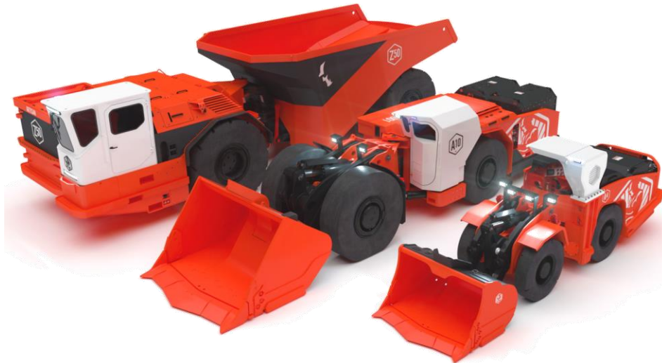
Fig. 1 Artisan battery-powered haul truck and LHD loaders
