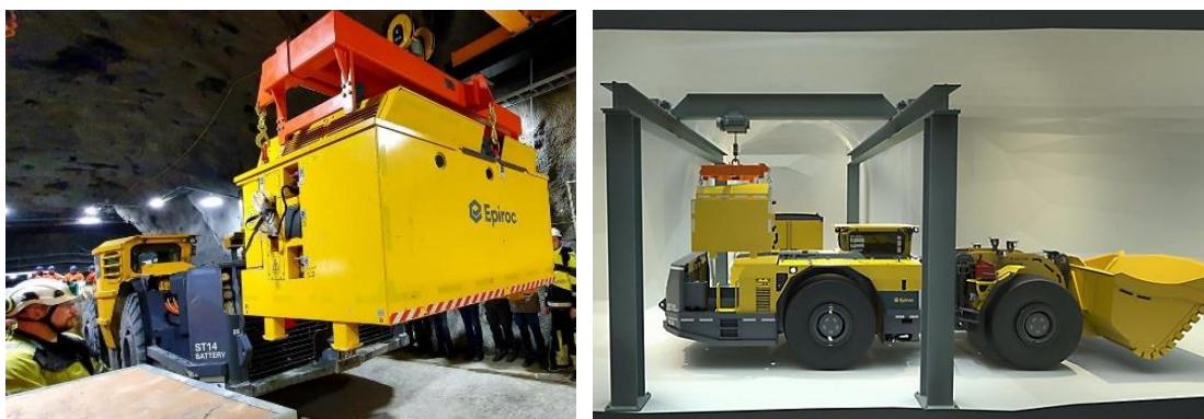
Fig. 6 Epiroc battery replacement system
