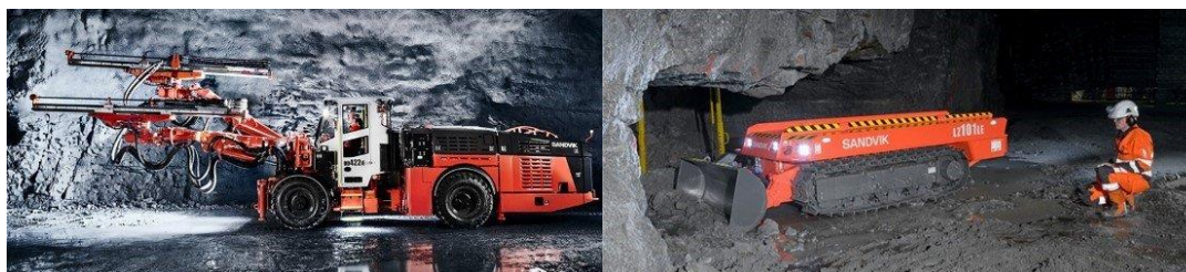
Fig. 4 DD422iE drilling rig and the LZ101LE ultra-low bulldozer produced by Sandvik
