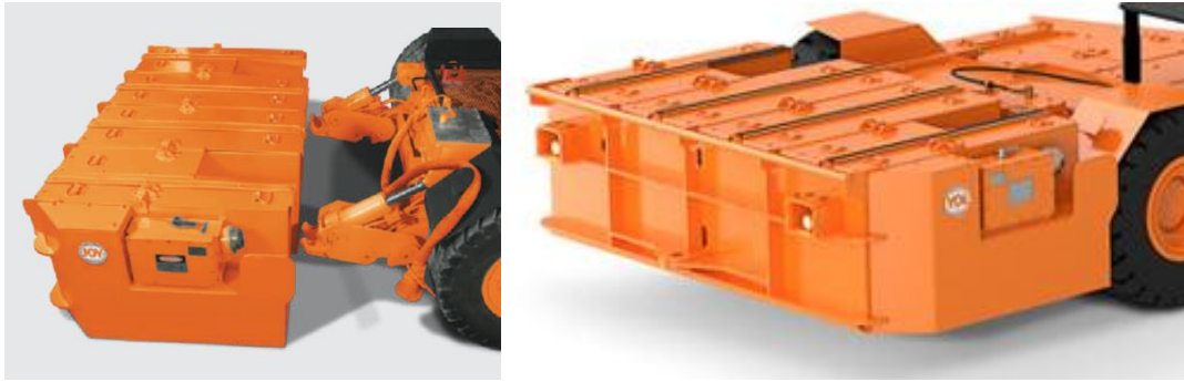
Fig. 8 Komatsu battery replacement system (Joy)
