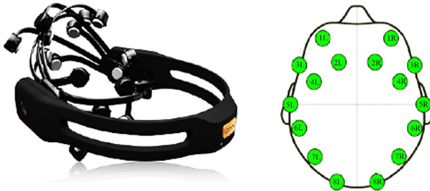
Fig. 4. Emotiv measurement interface and location of measurement points
