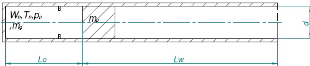
Figure 6. Physical model of the launcher system after opening of the gas flow from the pre-chamber to the projectile chamber – second period of the shot process.
