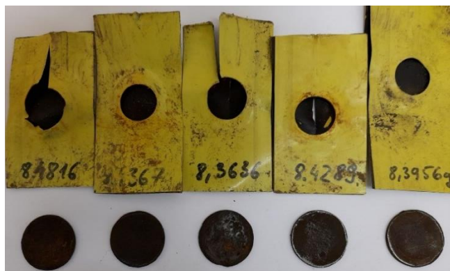
Fig. 5. Carbon steel samples after 4 years of exposure in the soil nearby to the main water tanks of Krakow water supply network
