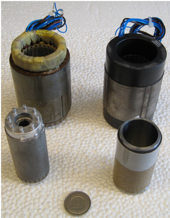
Fig. 1. Stator and rotor of a 3.4 kW induction motor/generator (left) and a 6-kW permanent magnet synchronous motor/generator (right) designed to operate at speeds above 80,000 rpm and voltage frequency above 1.3 kHz.
