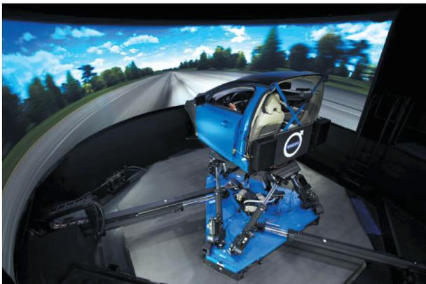
*Fig. 5. Volvo Dynamic Driving Simulator [6]*
