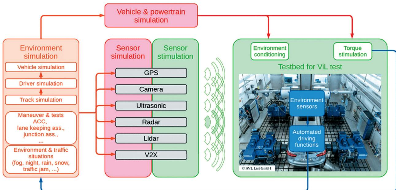
Fig. 14. Driving-Cube test bench for holistic testing of automated driving [27]
