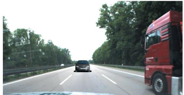
*Fig. 4. Real test drives augmented with virtual car [7]*
