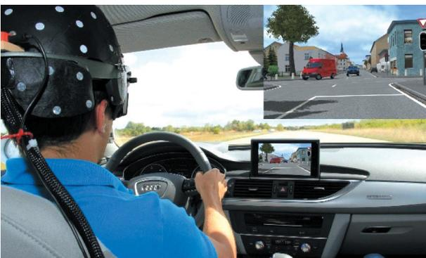
*Fig. 12. Real test drives augmented with virtual car [20]*
