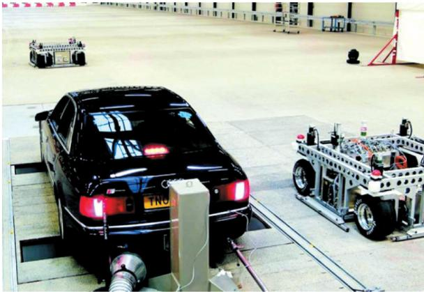
Fig. 13. Tested vehicle on the dyno with fake cars [23]
