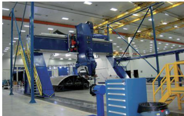
Fig. 8. Airbus A 350 fuselage panel manufactured with gantry style Electroimpact AFP machine [PF Products Finishing, 2015]
