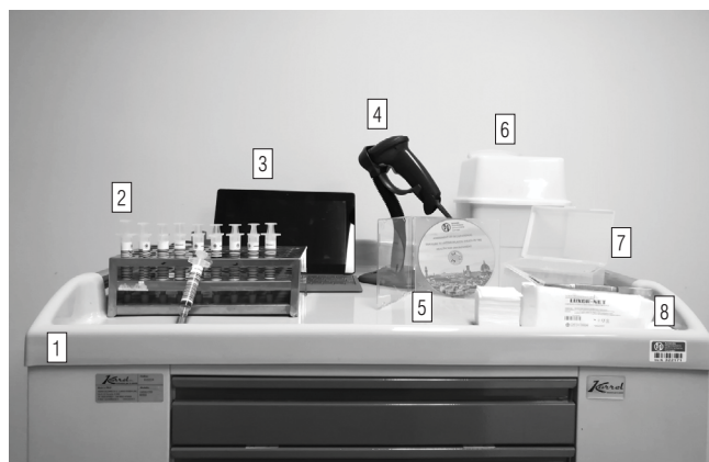
1 – wheel-trolley, 2 – 5-ml syringes, used for manual desorption, preassembled with 5×5 cm 3-layer nonwoven fabric and Combi Caps, 3 – personal computer, 4 – barcode reader, 5 – CD instruction manual with photos and a video on the correct technique for obtaining wipe samples, 6 – pipette tips waste container, 7 – pipette tips, 8 – 5×5 cm 3-layer nonwoven fabric and tweezers with joint for disposable pipette tips.
