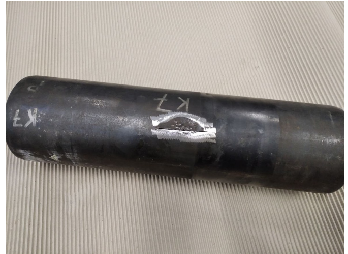
Fig. 2. Prepared point damage to the test roller tube
