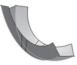
Fig. 31. Surfaces of worm wheel tooth space
