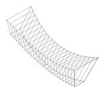
Fig. 27. Frame model of tooth space of worm wheel
