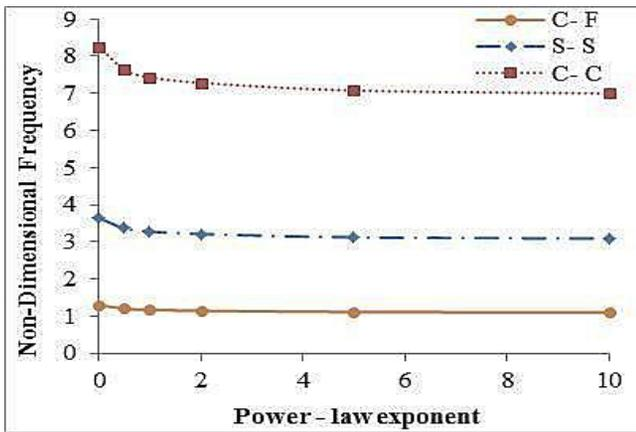
Fig. 7. Frequency of beams having different boundary conditions at slenderness ratio =100
