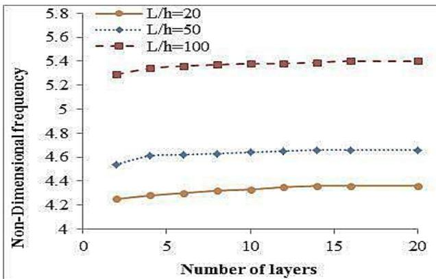
Fig. 8. Dimensionless essential frequencies of the sandwich beams for different layers numbers with various ratios of thickness at  $k=0.3$
