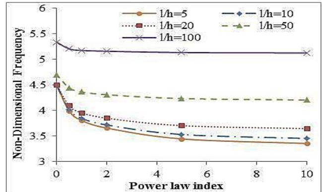
Fig. 5. Frequency parameter for S-S beam, face sheet thickness (2 mm)
