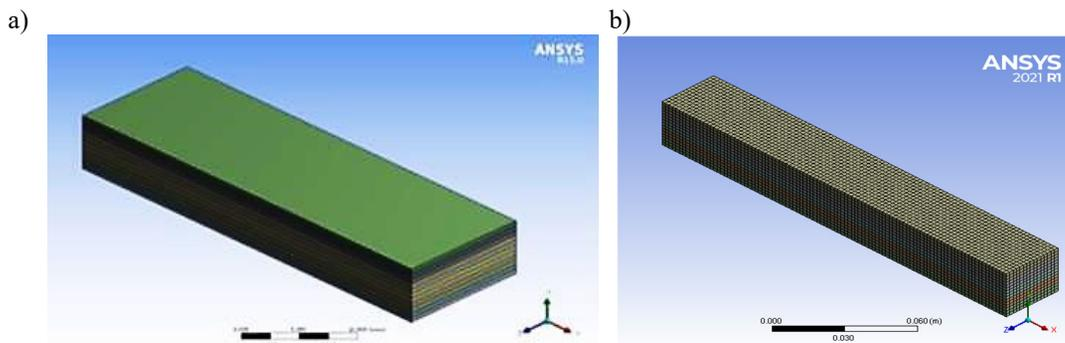
Fig. 3. The model of the FGM sandwich beam without (a) and with mesh (b)
