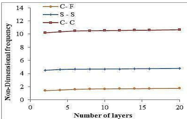
Fig. 9. Dimensionless essential frequencies of the FG sandwich beam various layers numbers with different thickness BC's at  $k=0.1$
