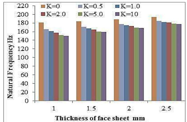
Fig. 6. Analytical results of the natural frequency of (S-S) beams at  $L/h=50$ , for various values of the power-law index
