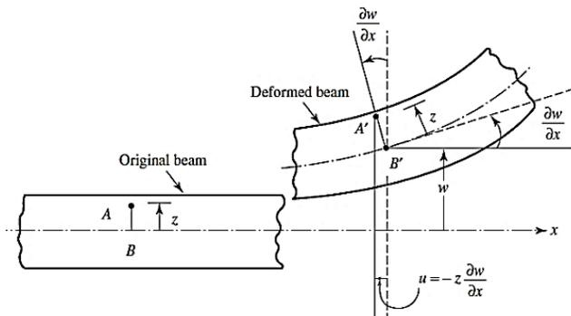
Fig. 1. The deformation of a distinctive transverse perpendicular line in CBT [34]
