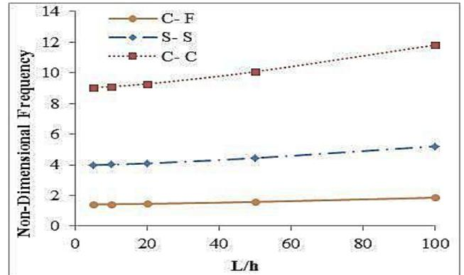
Fig. 4. Frequency parameter under various B.Cs. and at (2 mm) face thickness and  $k=0.5$
