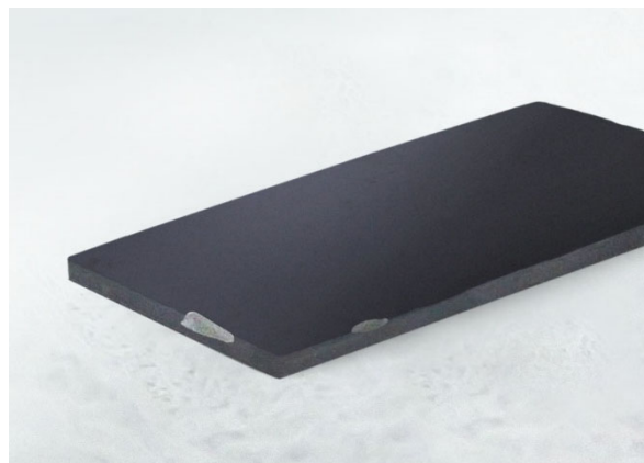
Fig. 5. Example of a defective sample from batch 3 (orientation (111), impurity concentration 1.2 \times 10^{19} \text{ cm}^{-3} ): on the surface you can see a chip formed as a result of improper use of the sample and due to the fragility of the plate
