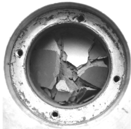
Fig. 5. Briquette destroyed as a result of an outburst induced under laboratory conditions
