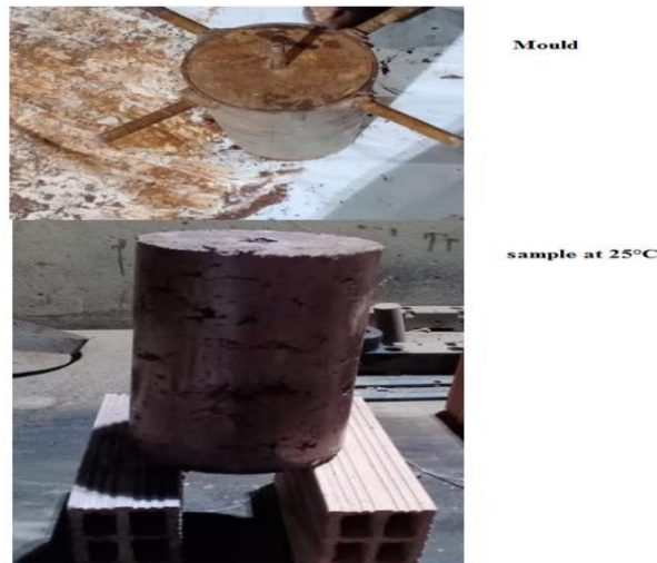
Fig. 3. Photograph of samples of clay doped by reed plant fibers at 25°C
