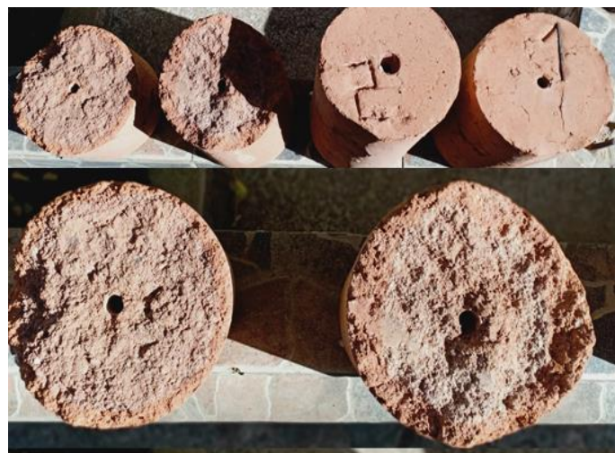
Fig. 4. Photograph of red brick doped by reed plant fibers at 825°C
