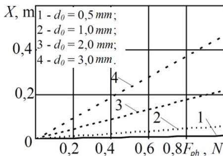
Fig. 4. Graphs of change in the distance  $X$ , by which it is necessary to move the chip element along the slot as a function of the force of forced pneumatic hydrodynamic impact  $F_{ph}$  during machining steel blanks with a solid cutter made of high-speed steel
