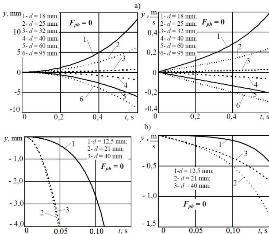
Fig. 3. Graphs of changes in the distance  $y$  and  $\dot{y}$  the speed of movement of the chip element along the front surface of the cutter tooth as a function of time  $t$  for a solid cutter made of high-speed steel during processing: a) steel ( $F_{ph} = 0$ ); b) cast iron ( $F_{ph} = 0$ )
