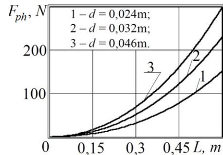
Fig. 5. Graphs of the dependence of the required force of forced pneumatic hydrodynamic impact on the length of the body of drawing (with variable values of the cutter diameter)
