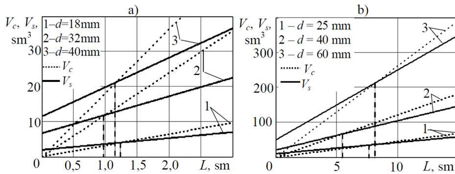
Fig. 2. Graphs of the change in the volumes of the separated the chip  $V_c$  and the slot space  $V_s$  as a function of the cutter displacement  $L$ : a) for a solid cutter made of high-speed steel during milling steel ( $v = 25$  m/min;  $f_z = 0.05...0.12$  mm/tooth); b) for a cutter with brazed carbide inserts during milling cast iron ( $v = 55...40$  m/min;  $f_z = 0.03...0.06$  mm/tooth)
