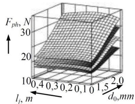
Fig. 6. Graphs of the change in the force of the jet action on the obstacle for the pressure values  $p_0 = 2; 3; 4; 5 \text{ MPa}$
