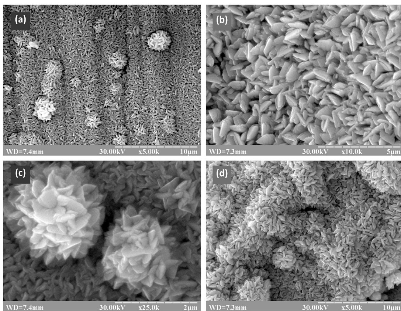
Fig. 3. SEM images of a sample treated on anode for 1 h in oxygen plasma (490 Pa, 600 V and 0.08 A): a) general view of a surface covered with the nanostructures; b) magnified view of the 2D nanostructures with the sizes of about  $500 \times 100$  nm; c) magnified view of the flower-like microstructures composed of the disk-shaped nanostructures; d) fragment of the surface showing the different morphologies composed of the same nanostructures
