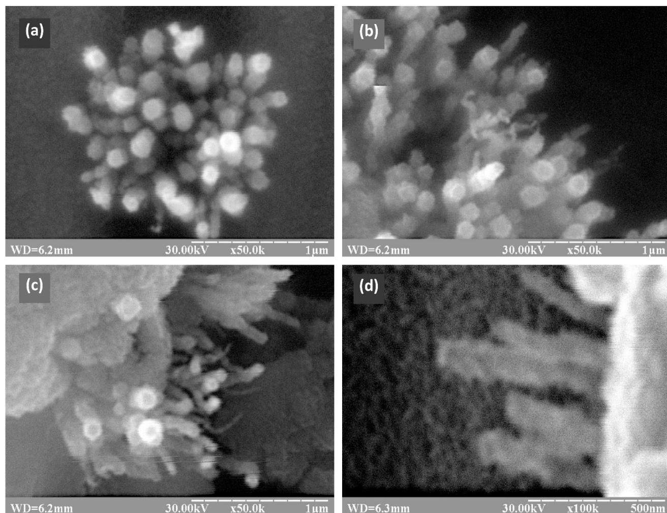
Fig. 4. SEM images of a sample treated on anode for 30 min in oxygen plasma (150 Pa, 600 V and 0.04 A): a) anemone-like nanostructure composed of nanowires; b) magnified view revealing the sizes of 1  $\mu\text{m}$  in length and 100 nm in diameter; c) same nanostructures but with a diameter of 50 nm; d) magnified view of the nanowires
