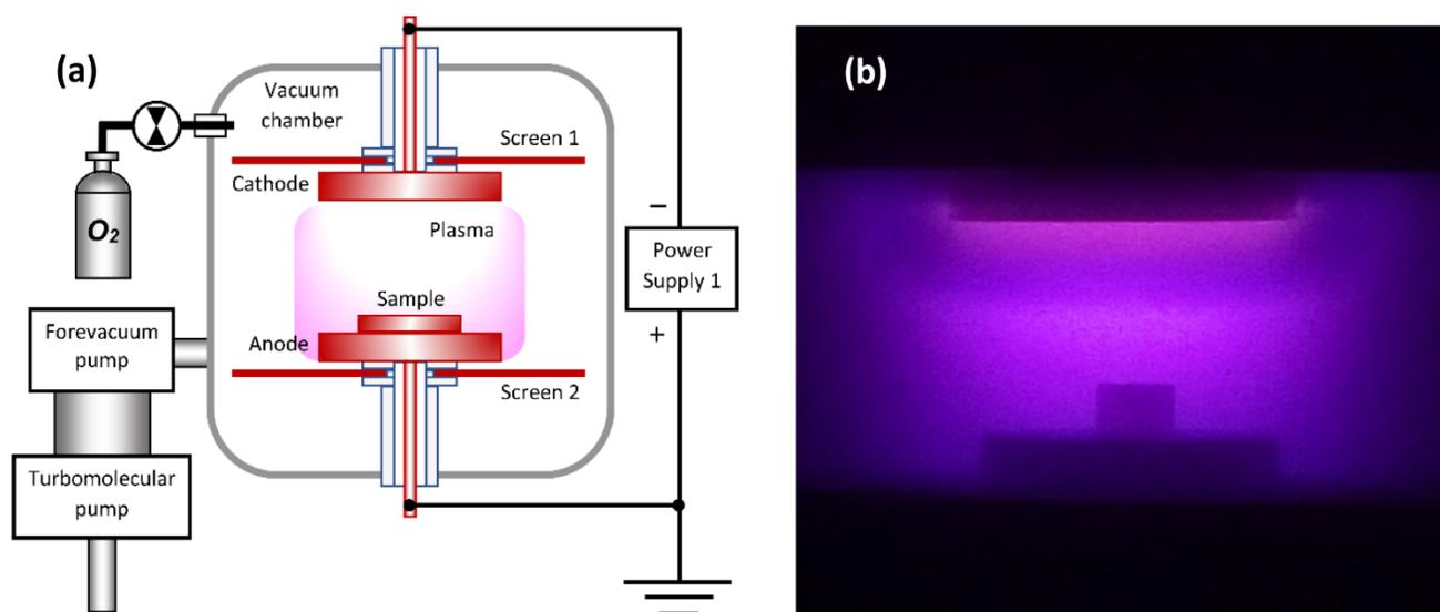
Fig. 1. Growth of copper oxide nanostructures in glow discharge: a) a schematic of the experimental setup, when a copper sample is installed on the anode; b) a photograph of the glow discharge
