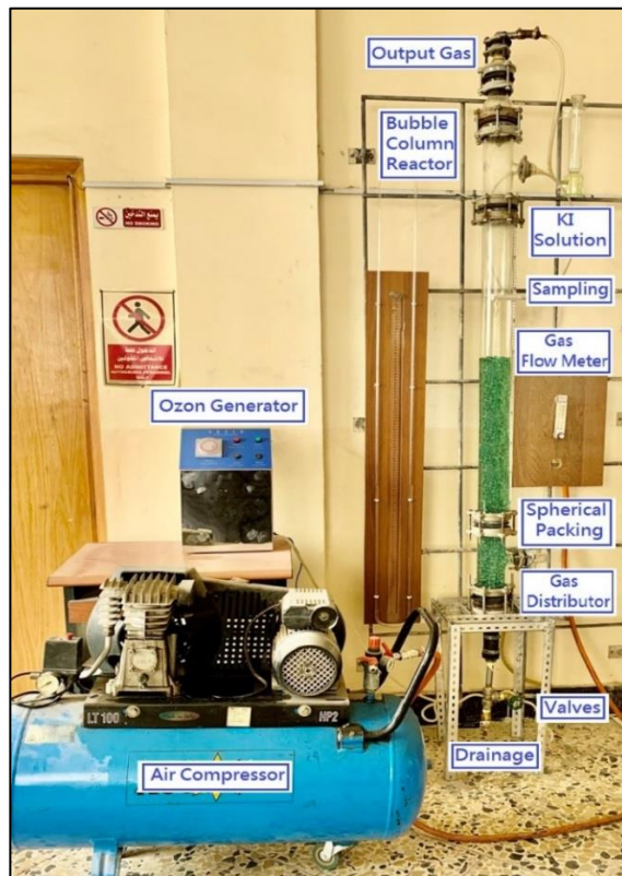
Figure 1. The experimental apparatus of packed bubble column reactor. Source: Author
