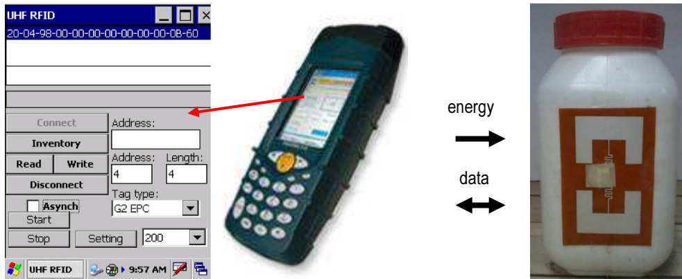
Fig. 6. The visualization of reading of electronic product code during the measurements of MRD.
