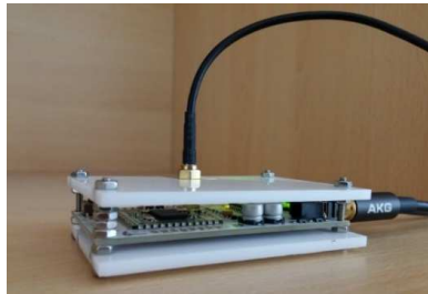
Fig. 3. Operating programmable DAB+ receiver.
