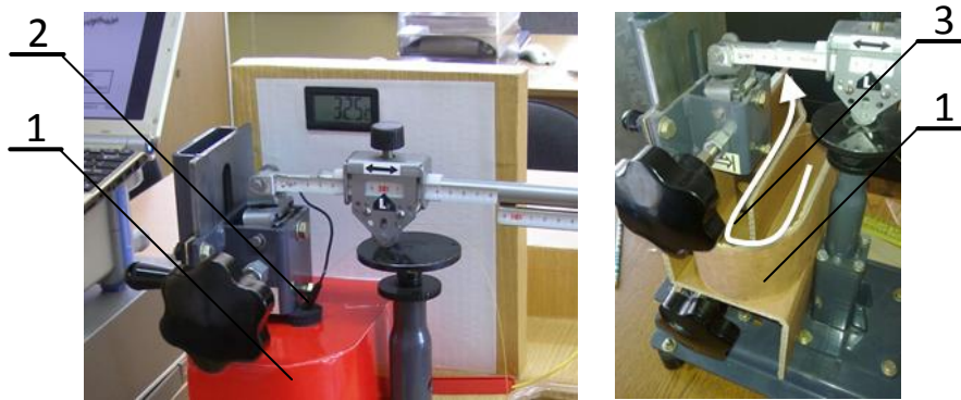
Fig. 2. Thermal chamber providing strain measurement in various temperature conditions: 1 - chamber enclosure, 2 - thermometer probe, 3 - flow direction of input air, with a regulated temperature.
