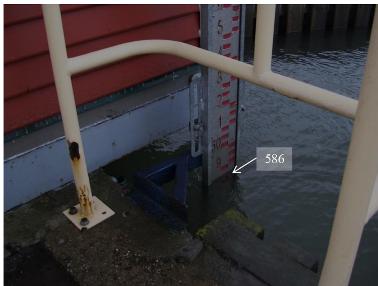
Phot. 1. Nearly the highest sea level (586 cm) observed at station Gdynia on 28 th November, 2016 [photo C. Dyrzcz]
