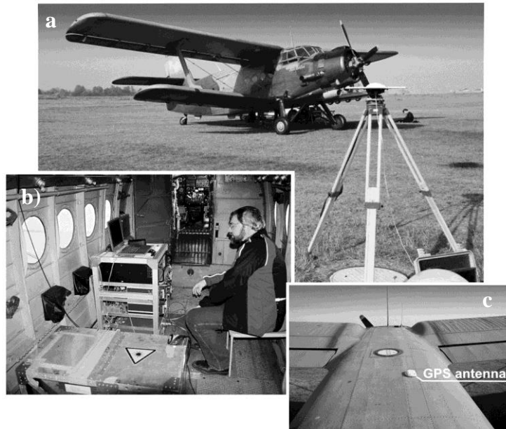
Fig. 3. a) AN-2 airplane and one of GPS reference station, b) scanner and control unit inside of airplane, c) airborne GPS antenna
