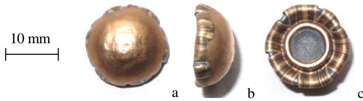
Fig. 3. Projectile after ballistic test: a - front, b - side, c - back
