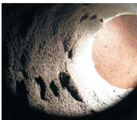
Figure 12. Deposits left in the position, before serving additive EKOSTABIL.
