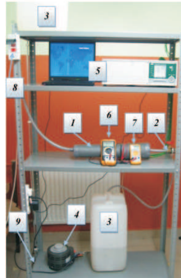
Figure 9: Thermal flow meter test stand: 1 – mass flowmeter, 2 – valve, 3 – water container, 4 – autotransformer, 5 – data acquisition system, 6 – ammeter, 7 – voltmeter, 8 – switch, 9 – pump.
