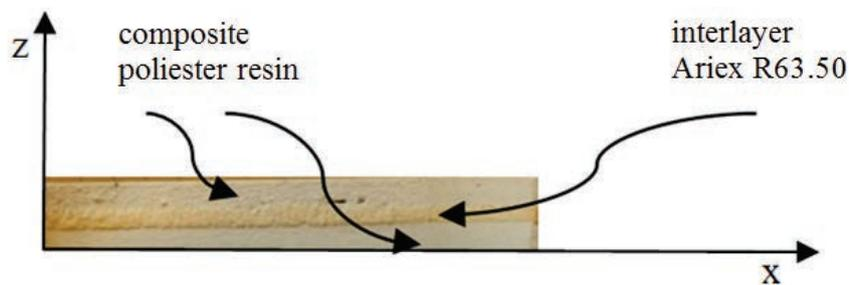
Rys. 4. Composite made of polyester resin and Ariex R63.50
