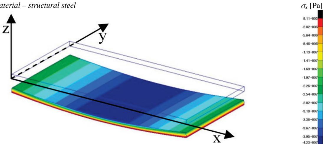
Fig. 5. Stresses distribution  $\sigma_x$  in the central part of the beam subjected to bending
