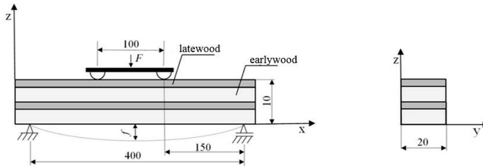
Fig.3. Support and load system of a beam
