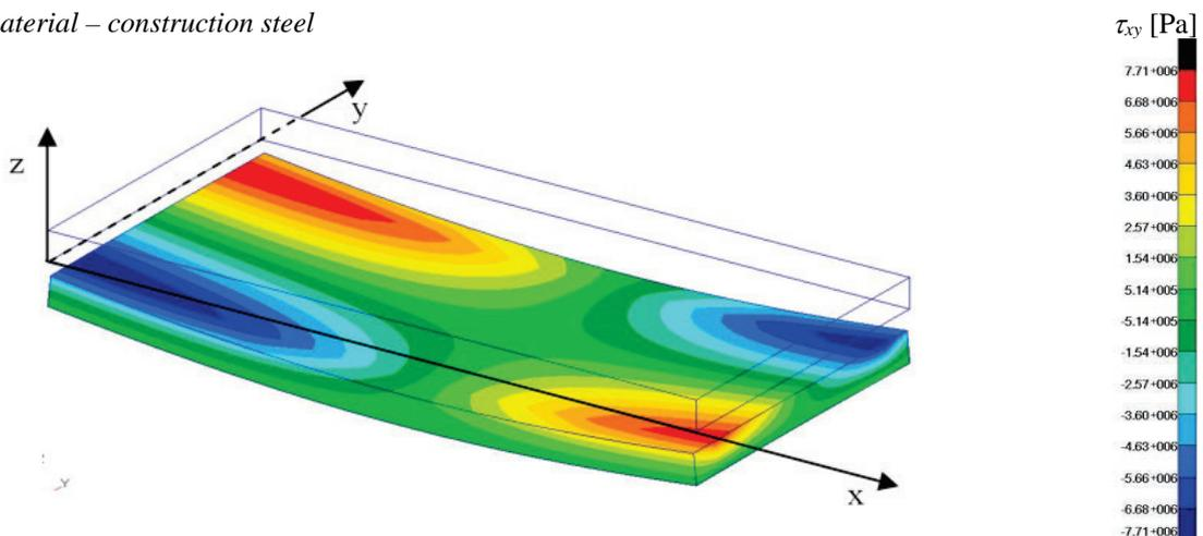
Fig. 6. Distribution of the shear stresses  $\tau_{xy}$  in the central part of a beam subjected to bending in a) wood, b) composite, c) steel
