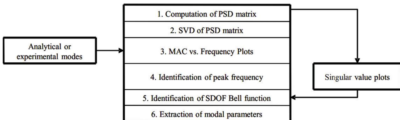
*Fig. 4. The algorithm for automated modal identification [6, 9]*
