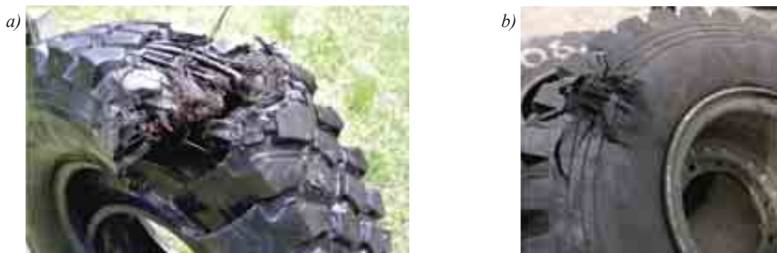
Fig. 7. Failures on the tyre following the crash into the IED: results of contact with IED (a) and results of increased pressure inside the tyre (b) (photo: G. Motrycz)
