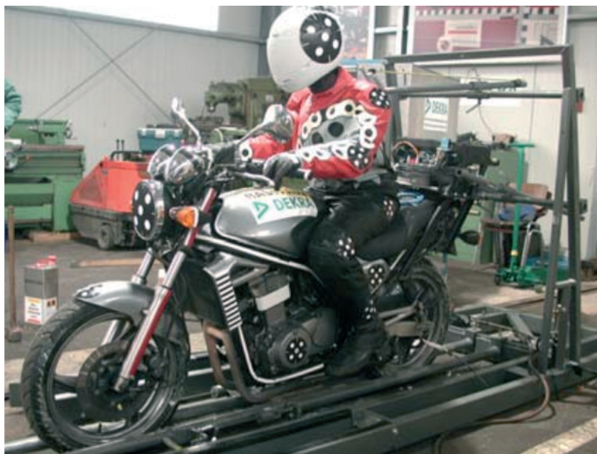
Fig. 18. Crash test bench with road barriers [19]
