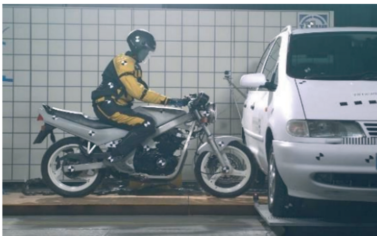
Fig. 16. Crash test recorded with a high-speed camera recording 1000 frames per second [14]
