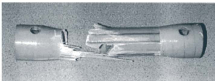
Fig. 5. Broken femur of the MATD dummy during the crash test [7]
