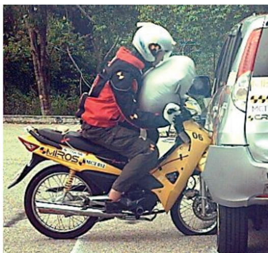
Fig. 12. Collision of a motorcycle with a passenger vehicle according to ISO 13232 – configuration 413 [24]
