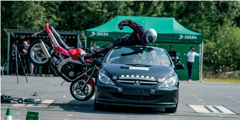
Fig. 6. Motorcycle crash test bench [18]
