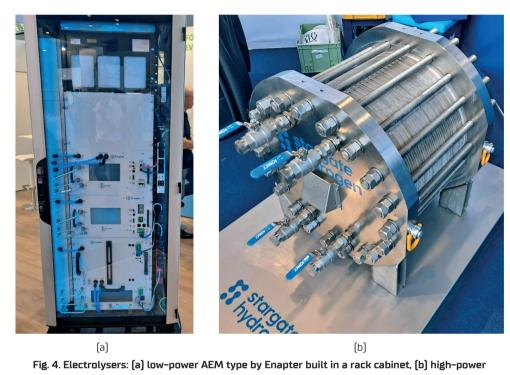
alkaline one by Stargate Hydrogen
