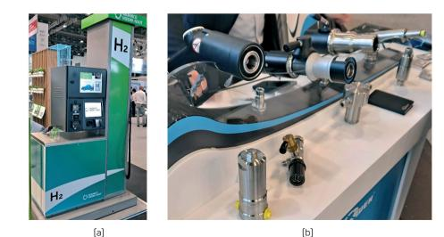
Fig. 17. Hydrogen refuelling technologies: (a) Gilbarco Veeder-Root hydrogen dispenser; (b) Weh hydrogen refuelling nozzles
