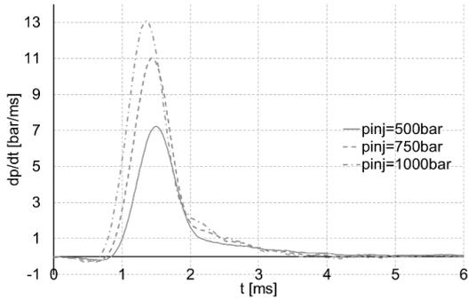
Fig. 10. ROPR ( $dp/dt$ ) for various injection pressure (fuel LFO, 70/590)
