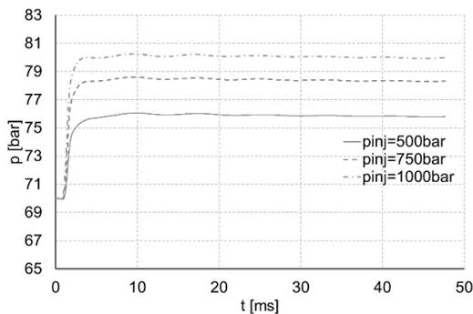
Fig. 8. Combustion pressure increase for various injection pressure (fuel LFO, 70/590)
