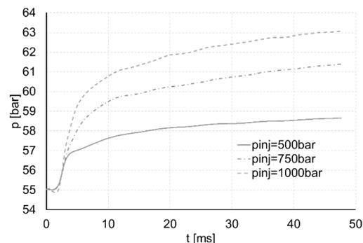
Fig. 4. Combustion pressure increase for various injection pressure (fuel LFO, 55/550)
