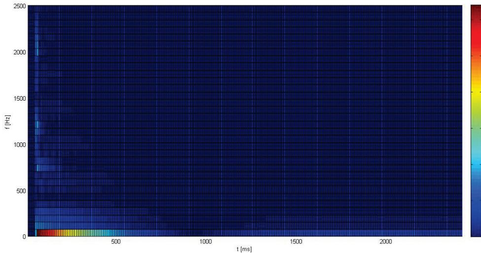
Fig. 1 Time-frequency dynamic characteristics 2D for a plate with no welded joints (0) for the impact made by an modal hammer with a metal head
