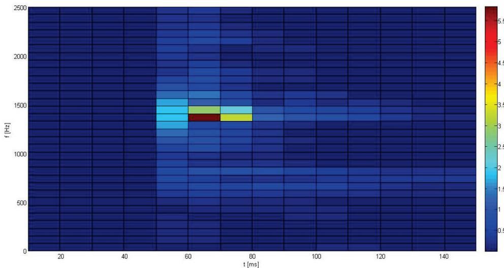
Fig. 2 Time-frequency dynamic characteristics 2D for a welded plate with non-defected welded joint (2202) for the impact made by an impact modal with a metal head
