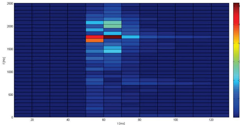
Fig. 3 Time-frequency dynamic characteristics 2D for a welded plate with a fault (lack of side fusion [2127]) for the impact made by impact hammer with a metal tip
