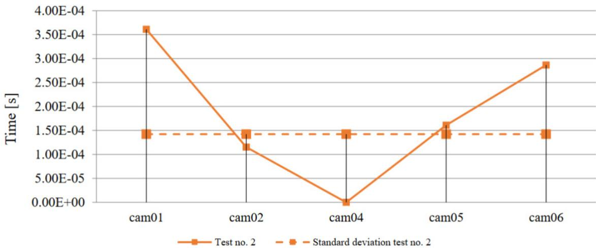
Fig. 7. The software trigger (solid line) time delay in reference to camera 4 with calculated standard deviation (dashed line)
