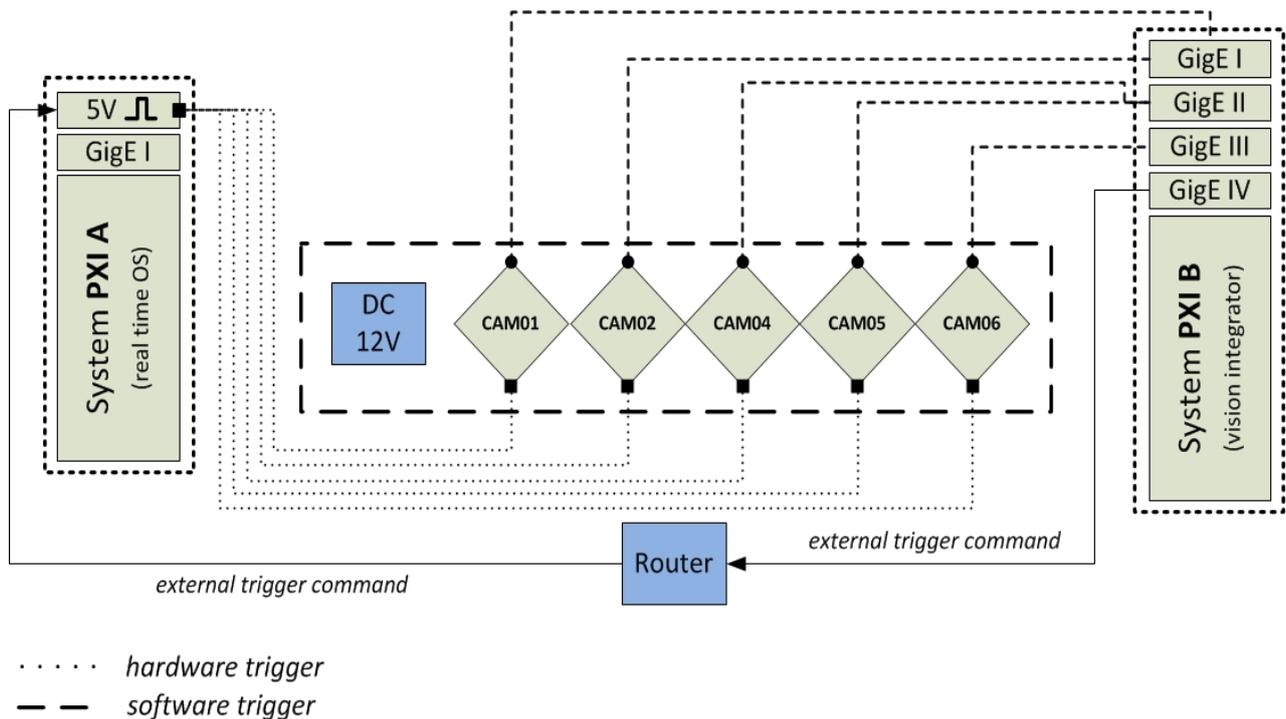
Fig. 1. The architecture to estimate hardware vs. software trigger time delay
