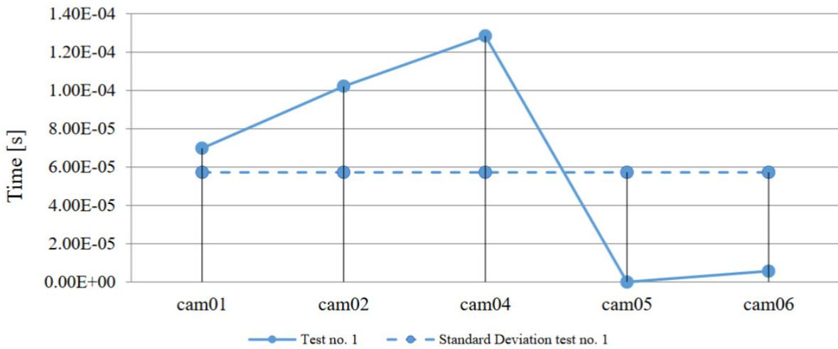
Fig. 6. The software trigger (solid line) time delay in reference to camera 5 with calculated standard deviation (dashed line)
