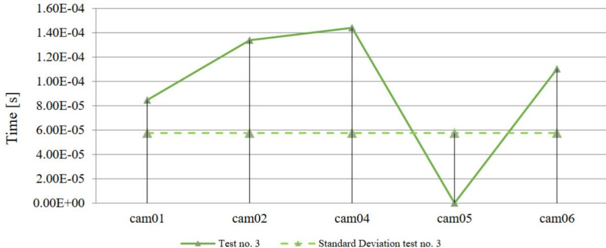
Fig. 8. The software trigger (solid line) time delay in reference to camera 5 with calculated standard deviation (dashed line)
