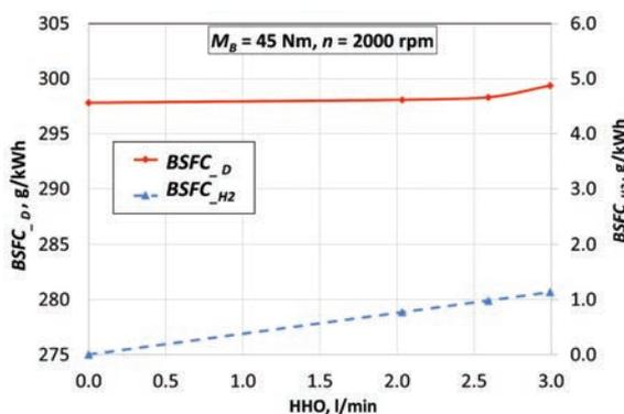
Fig. 4. HHO gas amount influence for Break Specific Fuel Consumption (BSFC)
