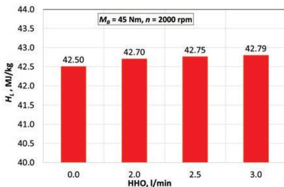
Fig. 2. The influence of HHO gas on the lower heat value of the mixture of fuels
