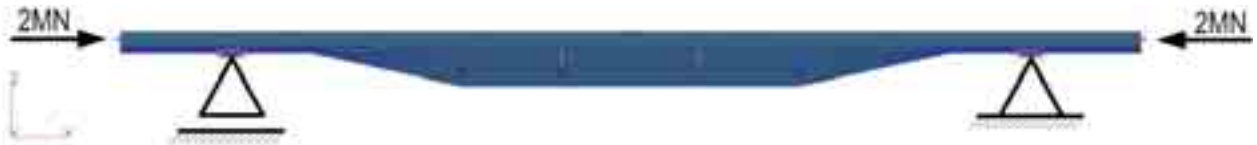
Fig. 6. Variant A: compression of the wagon in the axis of buffers with force of 2MN
