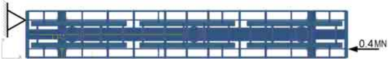
Fig. 7. Variant B: compression of the wagon with force of 0.4 MN applied diagonally on the level of buffers
