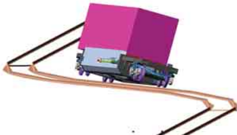
Fig. 12. Railway wagon overturning after reaching the first chicane
