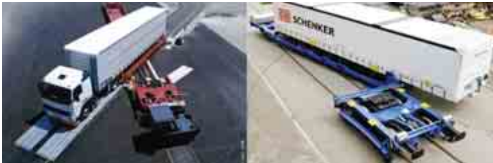
Fig. 1. Intermodal systems used in France: Modalohr (left) and in Sweden: Megaswing (right) [5, 6]
