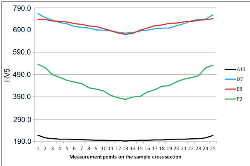
Fig. 5. Graphs of ball hardness obtained from 100Cr6 steel rolled in the modified method, cooled in three quenching media
