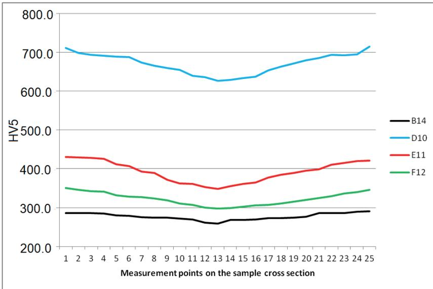
Fig. 7. Graphs of ball hardness obtained from steel cut from railway rail rolled in the modified method, cooled in three quenching media
