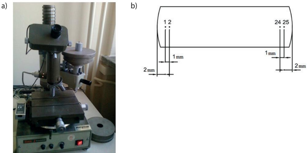
Fig. 3. Hardness measurements: a) hardness tester; b) scheme of points positioning on the length of the sample
