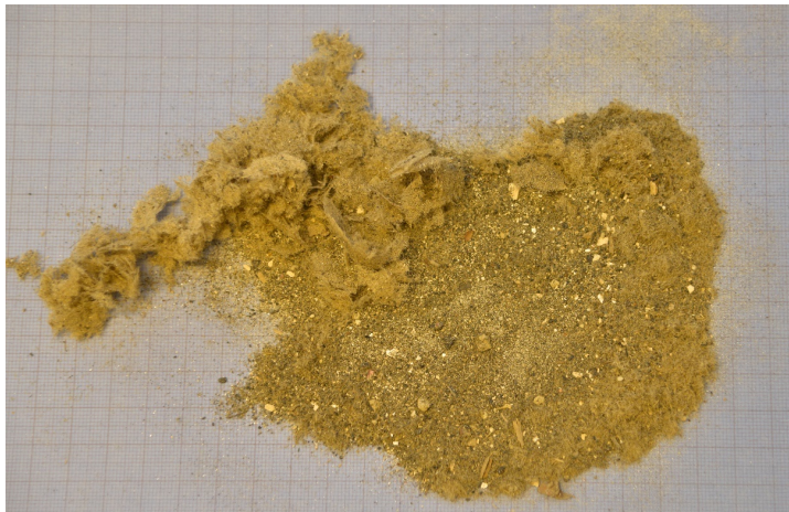
Fig. 3. Photo showing dried material after washing sieving. Note the amount of fibre at the top of the image. Photo by Per Lindh
