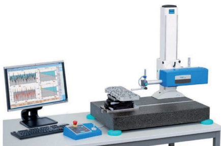
Fig. 11. Stand of surface topography measurement and areas in the die used for the measurement of surface topography
