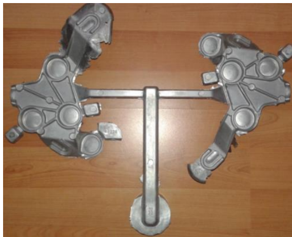
Fig. 7 Unprocessed pressure casting together with the inlet system
