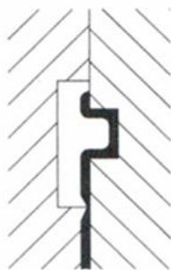
Fig. 14 Perpendicular component of momentum causing the filling of the segmented mold cavity shapes
