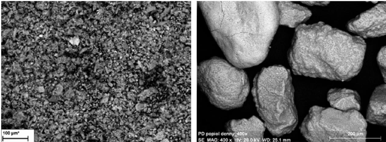
Figure 2. Microscopic photo of ashes (left-hand and right-hand side images are FA1 and BA, respectively)
