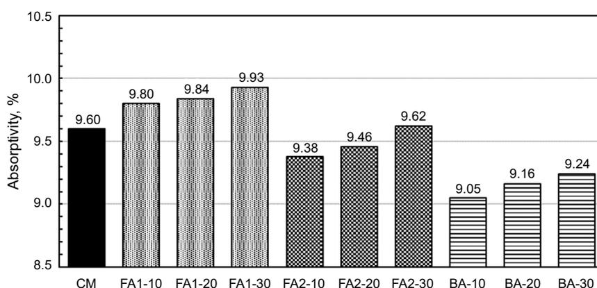
Figure 3. Water absorption of the cement mortars
