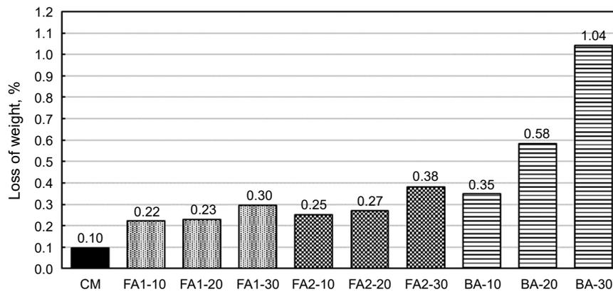
Figure 5. Weight loss after the frost resistance tests
