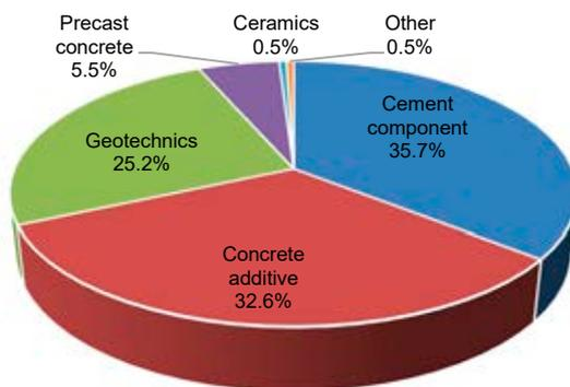
**Figure 1.** Use of waste ashes from the fuel combustion process conventional in Europe (Blissett & Rowson, 2012)
