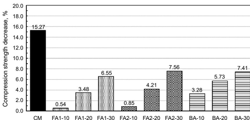
Figure 4. Drop in compressive strength after the frost resistance tests
