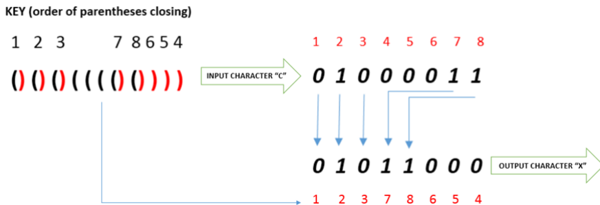
Figure 5. Encryption of character “C” in character “X”, based on Catalan-key K = ()()(((())()))
